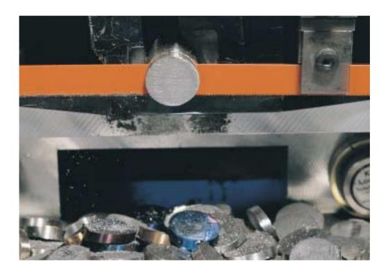
The New Sandflex cut 50 sections from the steel bar nearly 20% faster than its closest competitor. The New Sandflex blade also had the highest "MRR" value, that measures the removal of material from the workpiece in mm<sup>3</sup> per second.
